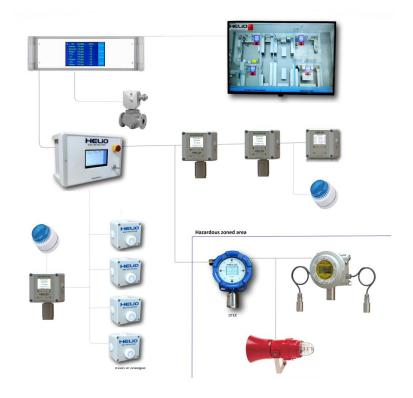
All Helio products can communicate with each other allowing a wide range of installations suiting most requirements with a single solution.
